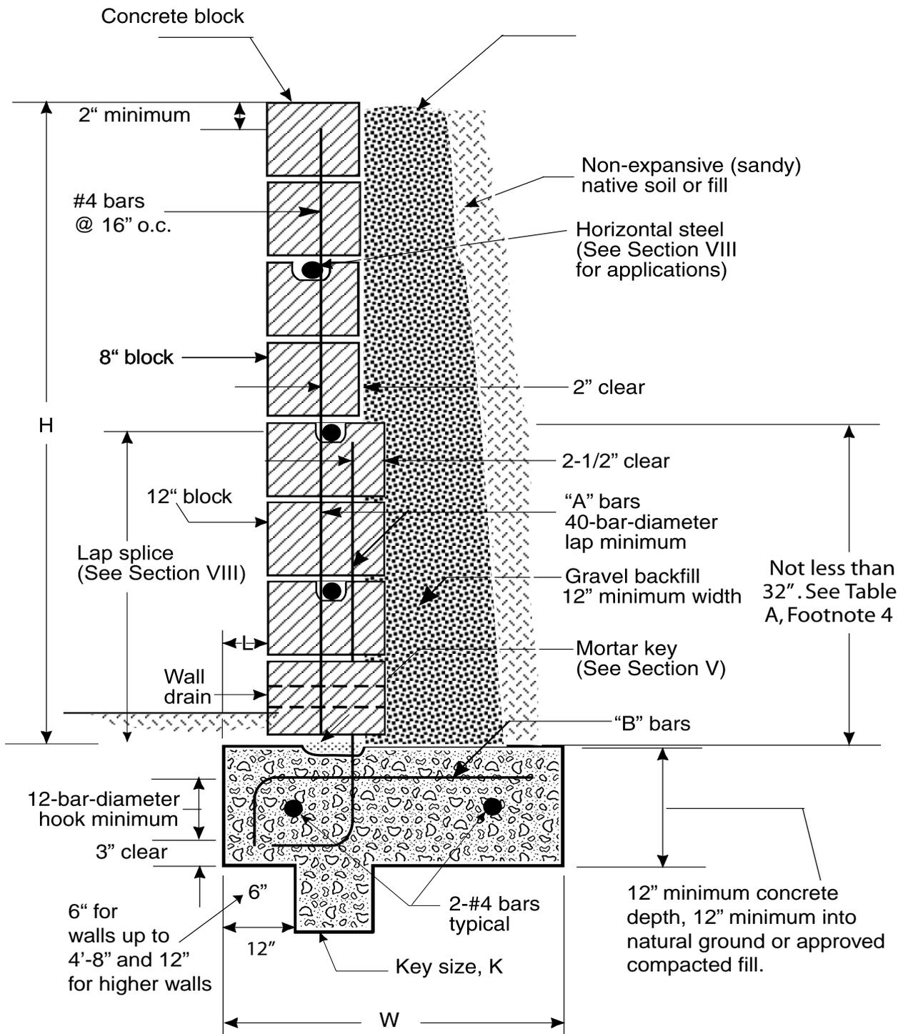
Note: A minimum of 7 feet must be provided horizontally from the toe of the footing to daylight where the ground slopes away from the base of the wall.
