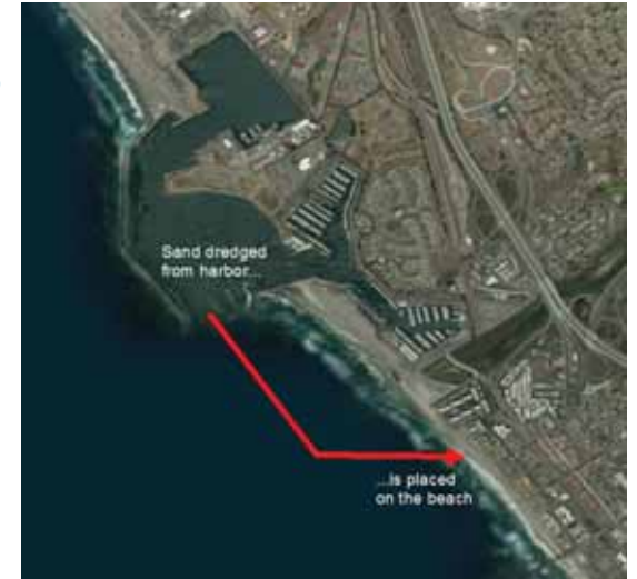
Sand bypassing concept illustration
