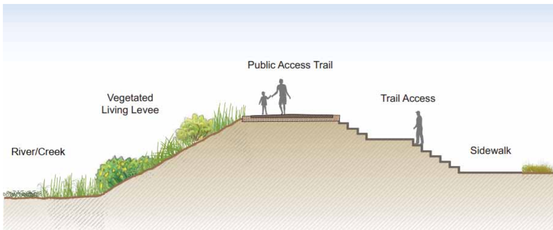
Levee Cross-section with Public Access
